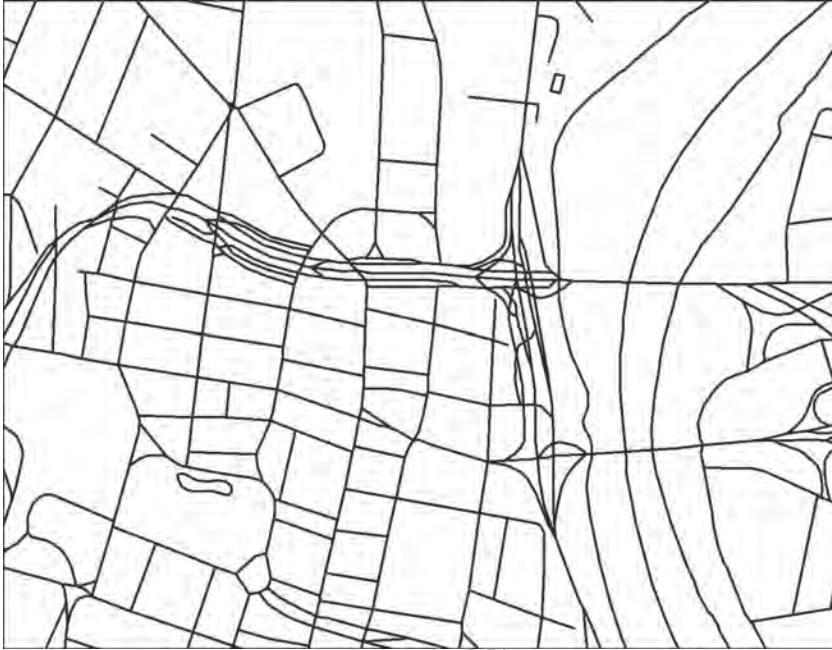
FIGURE 3.3. A portion of the 1:24,000 digital line graph database for the area around downtown Hartford, including roads, hydrographic features, and town boundaries. This figure shows roughly the same area as Figure 3.1.
